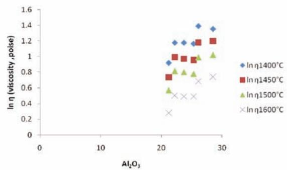
Fig.11. Effect of alumina on viscosity.
