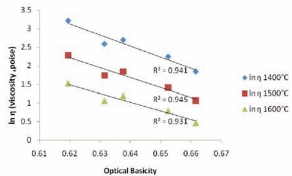
Fig.13. Effect of OB<sub>DUFFY</sub> on viscosity.
