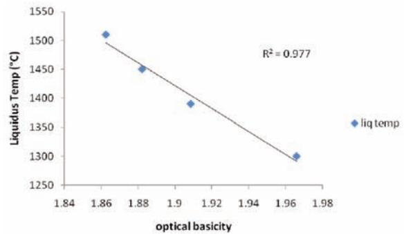
Fig.4. Effect of OB<sub>AS</sub> on Liquidus temp.
