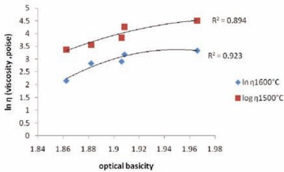
Fig.2. Effect of OB<sub>AS</sub> on viscosity.
