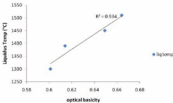
Fig.3. Effect of OB<sub>DUFFY</sub> on Liquidus temp.
