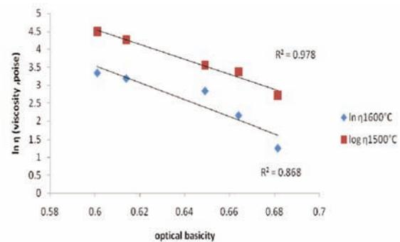
Fig.1. Effect of  $OB_{DUFFY}$  on viscosity.
