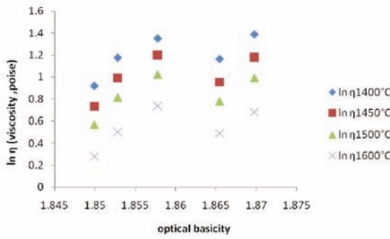
Fig.8. Effect of  $OB_{AS}$  on viscosity.
