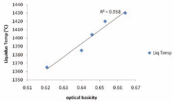
Fig.9. Effect of  $OB_{DUFFY}$  on Liquidus temp.
