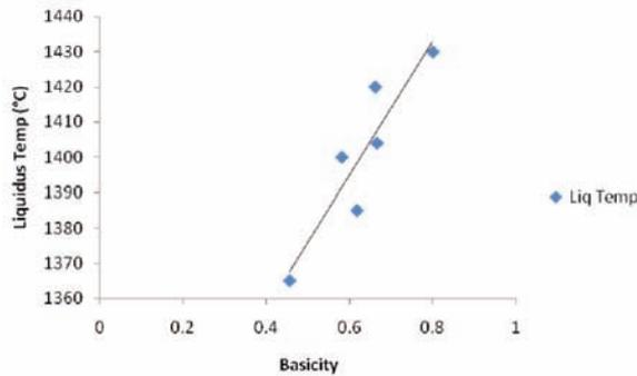
Fig.10. Effect of Basicity on Liquidus temp.
