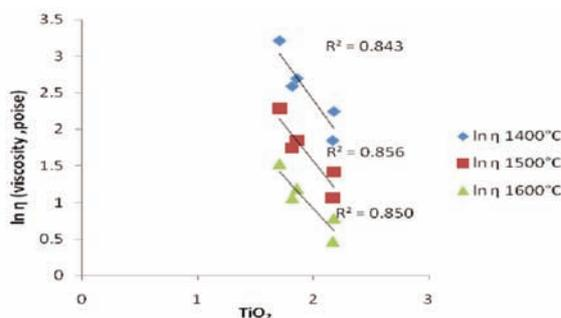
Fig.12. Effect of TiO<sub>2</sub> addition on viscosity.
