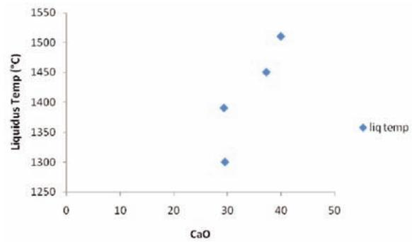
Fig.6. Effect of CaO on Liquidus temp.
